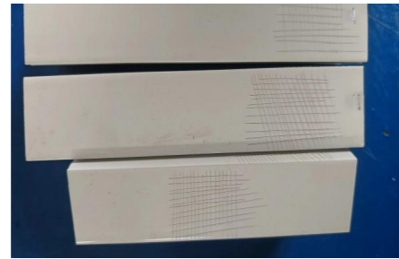
干湿附着检测 Dry and wet adhesion testing
