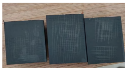
干湿附着检测 Dry and wet adhesion testing
