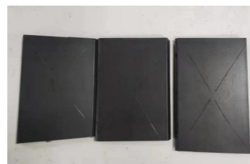
1000h ASS盐雾检测 1000h ASS salt spray detection
